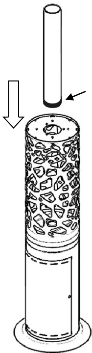
Figure 3— Placing the tubular glass
